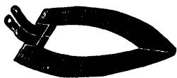
FIG. 77. — The fine wires are strongly heated by the current which flows through them.
